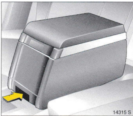
Demontage des Travel Assistant Untere Taste am Travel Assistant drücken.
